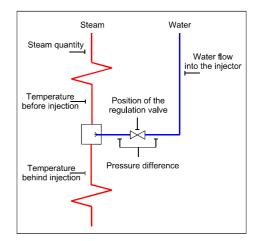
Using NID, it was diagnosed that the state of the injection valve was unsatisfactory as there was significant leakage, causing problems with reaching the temperature and with the quality of output steam temperature control (before repair). After repair, using NID methods again, the good condition of the valve was diagnosed – the repair had brought the expected result.
